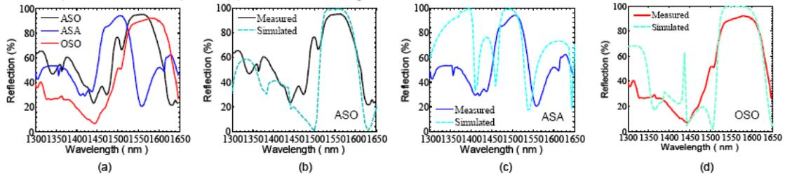
**Fig. 4** (a) Measured reflection for the same sample with three configurations: ASO (air-Si-oxide), ASA (air-Si-air) with 4 min BHF of ASO structure; and OSO (oxide-Si-Oxide) with SOG backfill of ASA sample; (b) to (d) Measured reflection results, along with the simulation (fitted) results for ASO, ASA, and OSO configurations.
