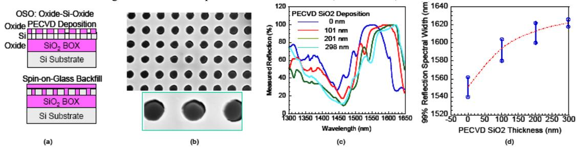
**Fig. 3** (a) Spectral trimming (Red-shift) with controlled SiO<sub>2</sub> coating with either PECVD deposition (top) or spin-on-glass (SOG) backfilling; (b) SEM images of Patterned SOI with SOG backfilling, showing the air holes filled with SOG SiO<sub>2</sub>; (c) Measured reflection characteristics with different SiO<sub>2</sub> thicknesses deposited on top of the patterned SiNM (from 0 to 298 nm); and (d) 99% reflection spectral widths for different PECVD oxide thicknesses.
