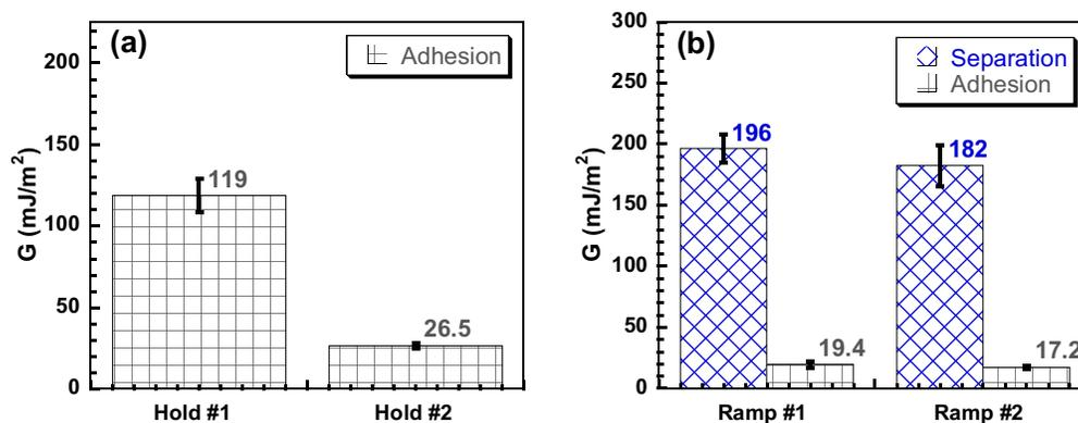
Figure 5. Results from tests conducted at  $\sim 50\%$  RH. (a)  $W_{adh}$  measured during the hold tests. (b)  $W_{sep}$  and  $W_{adh}$  values measured during the advancing and receding portions, respectively, of the ramp tests.
