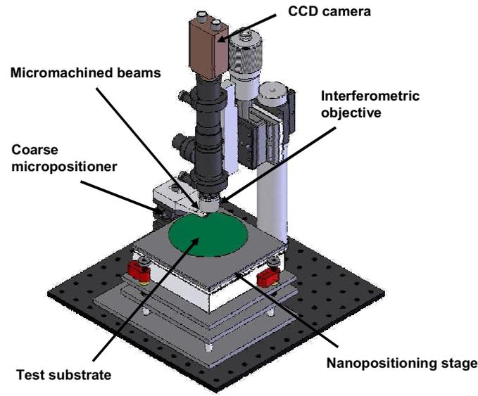
Figure 1. Test apparatus, with key components marked.
