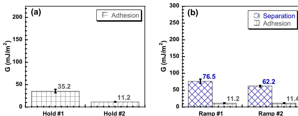
Figure 4. Results from tests conducted at  $\sim 15\%$  RH. (a)  $W_{adh}$  measured during the hold tests. (b)  $W_{sep}$  and  $W_{adh}$  values measured during the advancing and receding portions, respectively, of the ramp tests.
