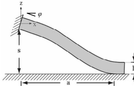
Figure 2. Schematic of a deformed beam in adhesive contact with a test substrate. The separation gap ( $s$ ) is varied and the crack length ( $a$ ) is measured during testing.
