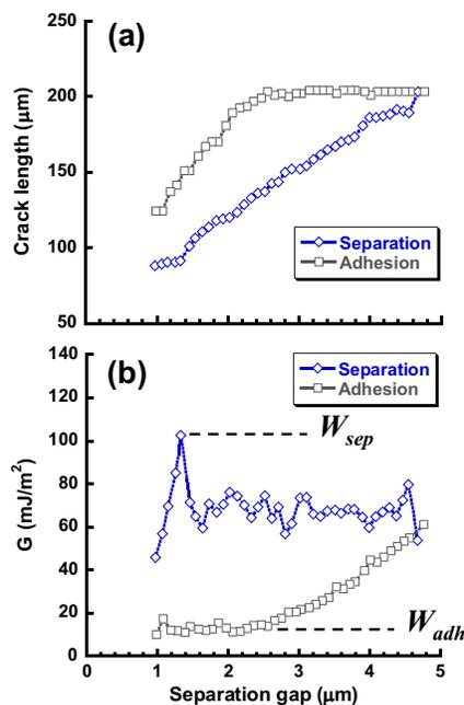
Figure 3. Example results from a test conducted at  $\sim 15\%$  RH in a nitrogen background. (a) Crack length versus separation gap. (b) Calculated values of  $G$  corresponding to the data shown in (a).
