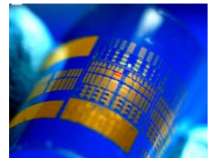
Figure 2. Image of an array of lateral PIN diodes made from Ge nanomembranes to make a flexible photodetector. From Ref. 8.
