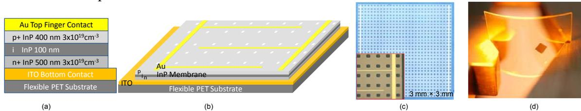
**Fig. 2** (a, b) Schematics of a InP p-i-n solar cell, based on transferred crystalline semiconductor nanomembrane processes; (c) A micrograph of a fabricated large area ( $3 \times 3 \text{ mm}^2$ ) InP solar cells on flexible PET substrate, with inset shown the zoom-in view of top finger contact; and (d) A close-up image of a fabricated crystalline flexible thin film solar cell on a bent PET substrate.
