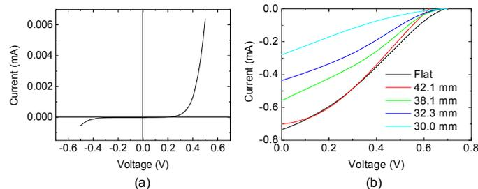
**Fig. 3** Measured flexible crystalline InP thin film solar cell characteristics: (a) Dark current; and (b) Currents at different bending radii, under standard AM solar simulator test conditions at room temperature.
