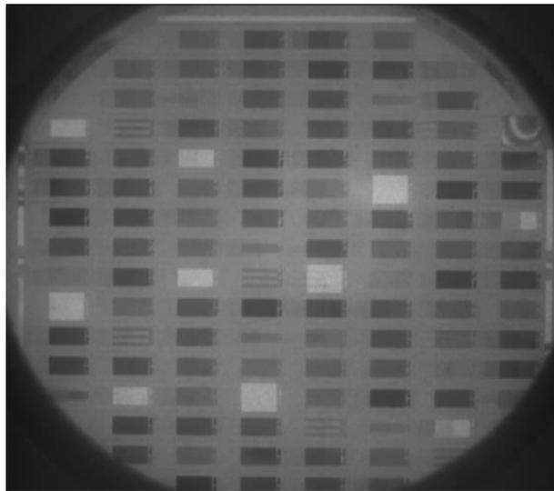
Figure 3. An example of IR inspection image of the bonded wafer pairs. The height of the pillars is 54  $\mu\text{m}$ . In this example, the overall bond quality is good except one specimen in upper right of the image where a fringe pattern is clearly visible.
