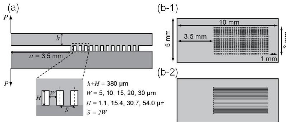
Figure 1. Geometry of the fabricated specimen. (a) sideview, (b-1) top view, (b-2) specimen with the line patterns used as a control “unpatterned” specimen. The specimen in (b-2) is used instead of a completely unpatterned interface as a control specimen to facilitate comparison to 2-D modeling results.
