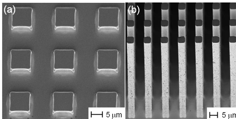
Figure 2. SEM micrographs of fabricated pillar structures: (a)  $H = 1.1 \mu\text{m}$ ,  $W = 10 \mu\text{m}$ , (b)  $H = 54.0 \mu\text{m}$ ,  $W = 5 \mu\text{m}$ .
