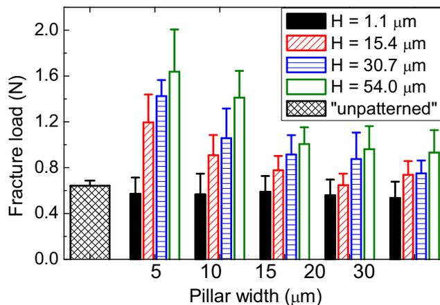
Figure 5. Results of the fracture load measurements. The fracture load values for the specimens with line patterns where lines are parallel to the crack propagation direction and the pattern height is 1.1  $\mu\text{m}$  are defined as the control “unpatterned” case.
