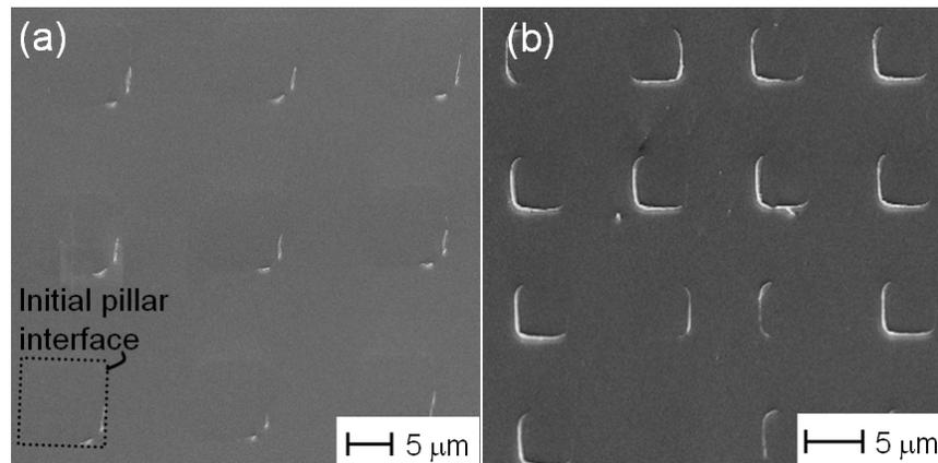
Figure 7. SEM micrographs of fracture surfaces of the specimens. These surfaces were flat and smooth prior to bonding. Original pillar geometries were (a)  $H = 1.1 \mu\text{m}$ ,  $W = 10 \mu\text{m}$ , (b)  $H = 54.0 \mu\text{m}$ ,  $W = 5 \mu\text{m}$ . Small parts of pillars fractured and remained on the surface after specimen failure. Still the crack propagates primarily at the interface. The crack propagated from left to right for both cases.
