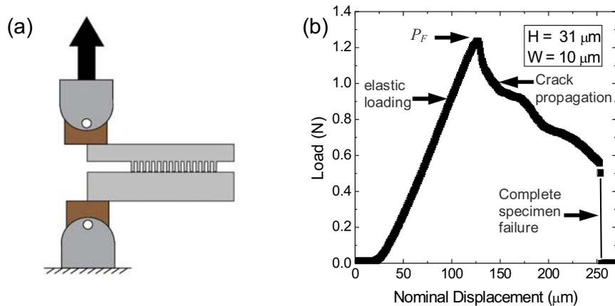
Figure 4. (a) Schematic of the fracture test setup, (b) a typical load – displacement plot showing the fracture load ( $P_F$ )
