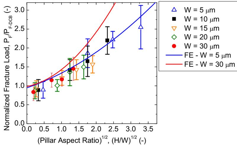
Figure 6. Normalized fracture load as a function of the square root of pillar aspect ratio obtained from experimental measurements. The experimental values are compared to the results from finite element simulations.
